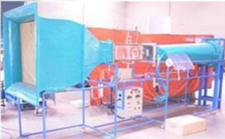
Subsonic Flow Wind Tunnel Test Setup
